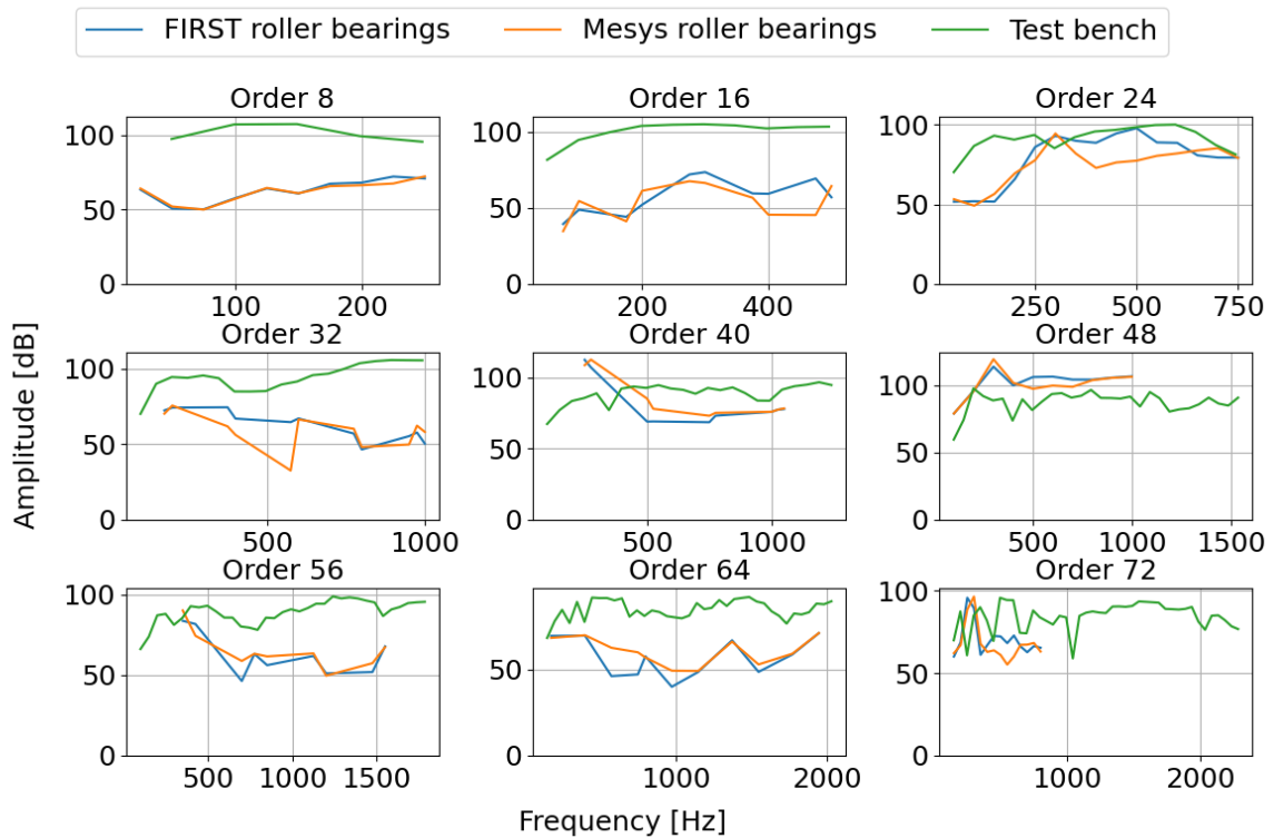
Figure 20: Order cut in spectrogram for one measurement point and comparison of roller bearing models with test bench data.
