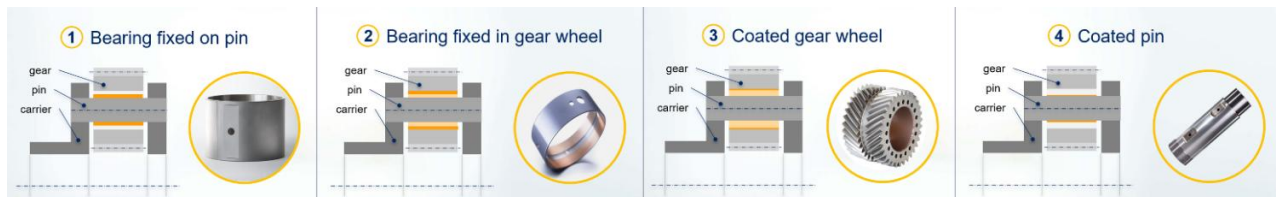
Figure 98: Support of planetary gear wheels by versatile HPB solutions. 1) Bushing with tribologically active material on the outer diameter, mounted on pin. 2) Bushing with tribologically active material on the inner diameter, mounted in gear wheel. 3) Direct coating of gear wheel. 4) Direct coating of pin.
