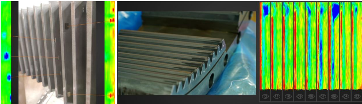
Figure 8: The distance-compensated measurement results of the automatic grinding burn test are shown as a false colour image. On the left are the measurement results for artificially introduced laser defects, on the right for tooth flanks with real grinding burn on the tooth tip (see etching image).
