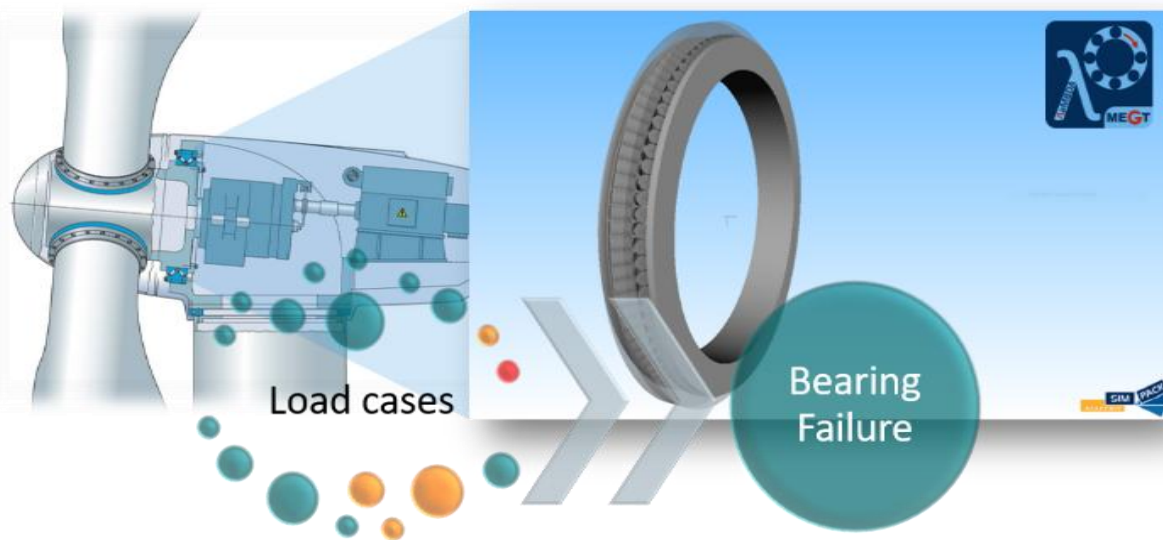
Figure 55: MBS model of a double row tapered roller bearing used as a main bearing in a multiple MW wind turbine modeled using LaMBDA
