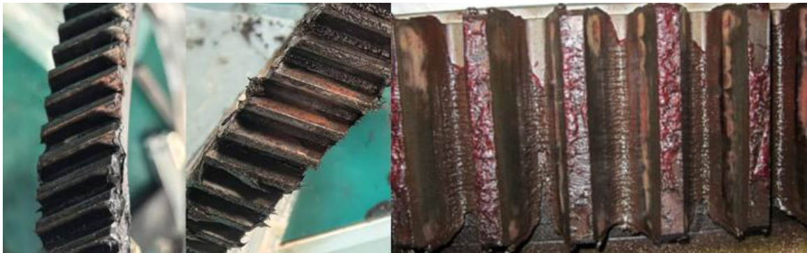
Figure 32 gear tooth surface appearance after test(left)/found in wind turbines(right)
