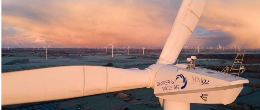
Figure 77: Wind turbine MM92 with two nacelle-based lidar systems. The right-hand lidar system (looking towards the rotor) was used in the following analysis.
