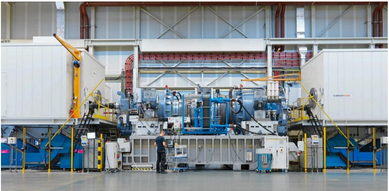
Figure 120: Back-to-back gearbox test rig at ZF Lommel. Installed gearboxes are illustrative and do not represent the gearbox instrumented in this paper.
