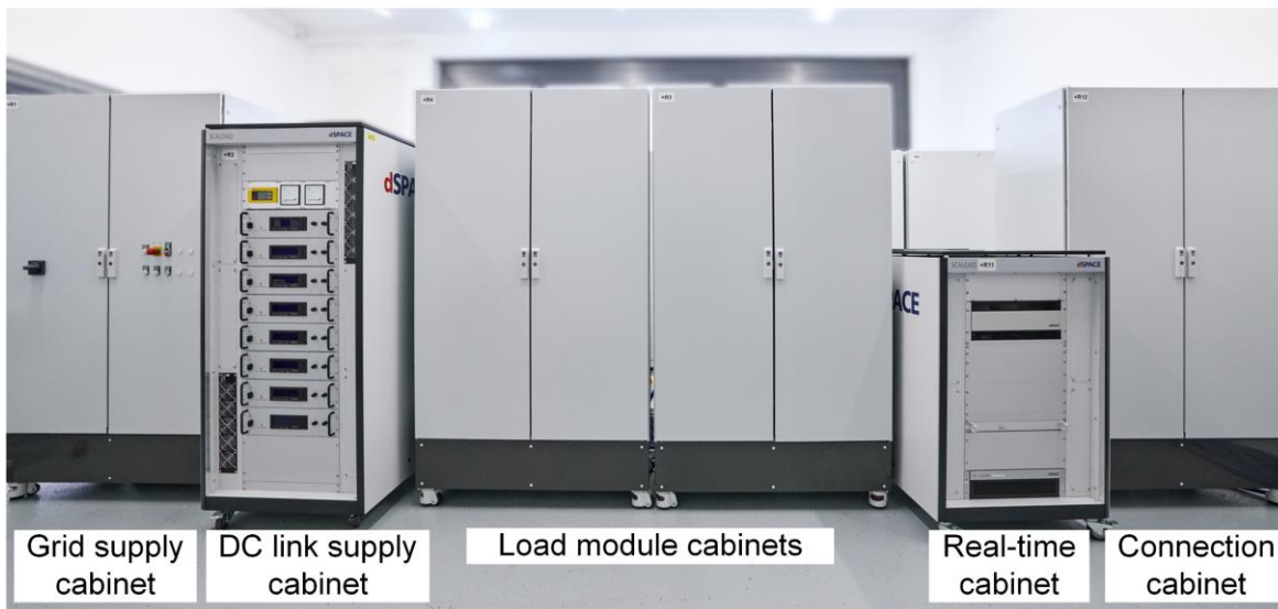
Figure 5: Setup of the entire component test bench in the laboratory
